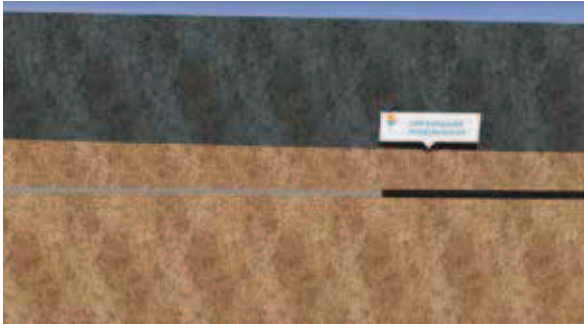
4. Pilot hole reamed (widened) and cable ducting pulled through from reception pit to drilling site
