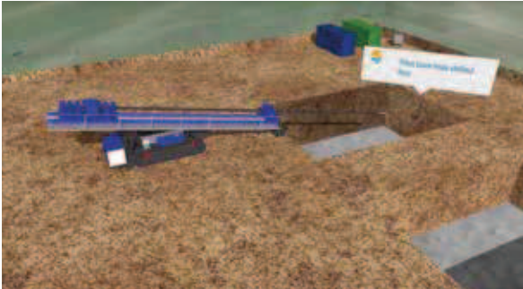
2. Excavation of joint pit, introduction of HDD rig and begin pilot bore
